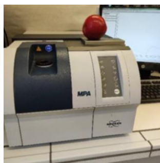
Fig. 1. FT-NIR spectrometer for recording the spectra of fruits.
